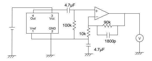
The cut-off frequency of HPF is approx. 0.3Hz and of LPF is approx. 1kHz.
