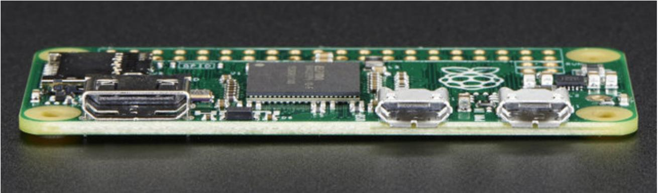
The most intriguing difference for hackers and makers is that the Pi Zero does not come with the soldered GPIO header. Partially this is to save cost, but it also allows the Pi Zero to be very thin and gives you the option of embedding it easily into a project box.
