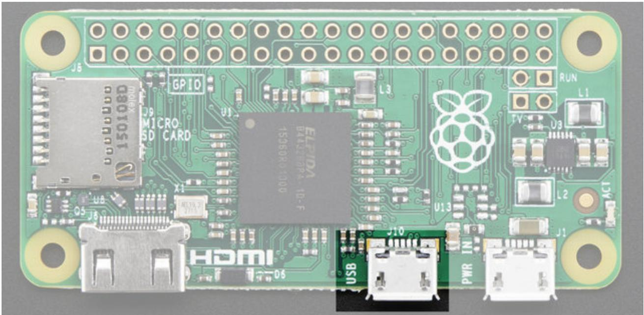
In order to connect a USB device (mouse, keyboard, WiFi) etc you'll need a [USB OTG micro B to A cable](http://adafru.it/1099) (<http://adafru.it/1099>):
