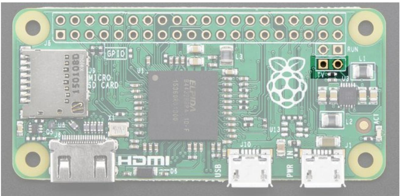
The hole on the left, nearest to the **TV** text, is the signal (+) line, the pin to the right of it is the ground (-) line. Solder two wires to these pads and connect them to an [RCA Jack](http://adafru.it/2792) (<http://adafru.it/2792>) like this one
